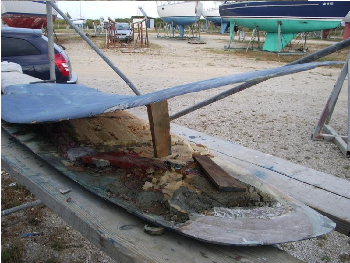
8 pics showing the splitting of the rudder – June 08
