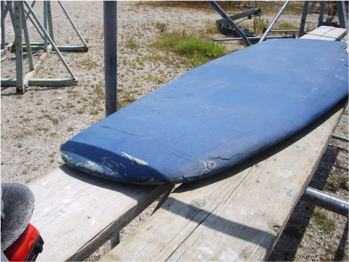
Rudder – now showing the hit spot in the front bottom– June 08
