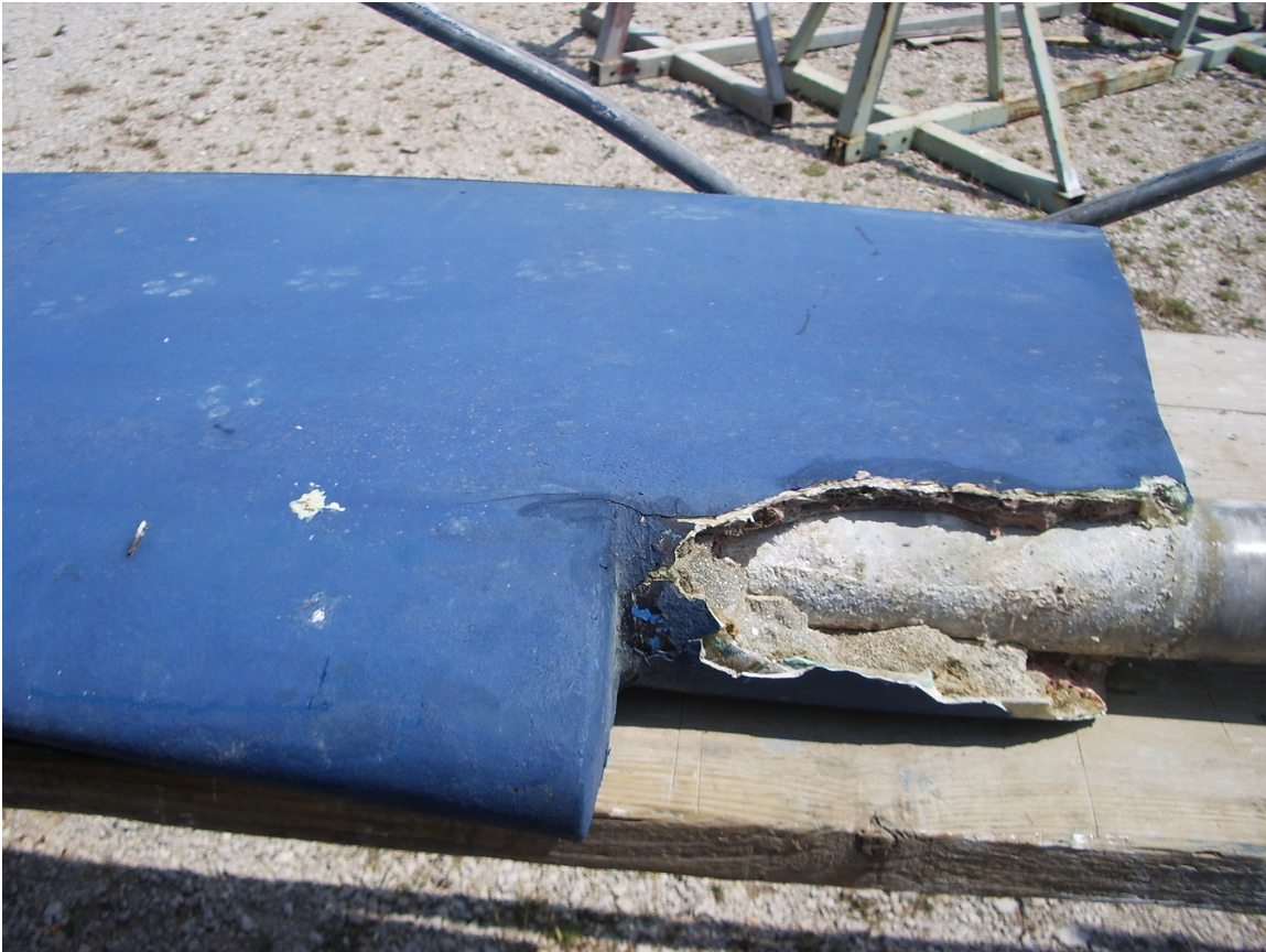
Rudder – now showing the main damage. – June 08
